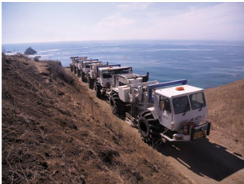
A wide-bin 3-D seismic survey using nodal technology system to better understand a promising Monterey oil prospect near Santa Maria, Calif., was successfully completed last year.
