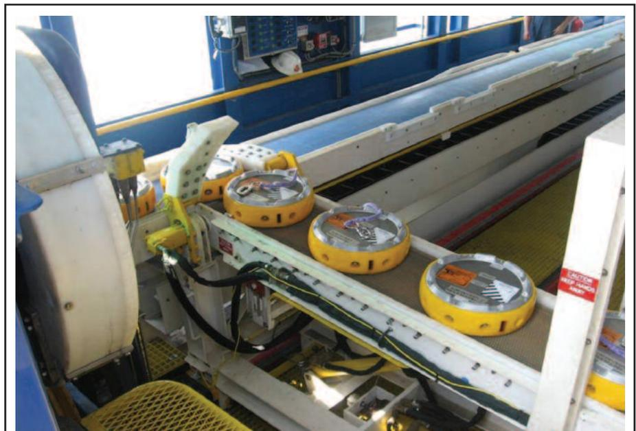
**Like all seismic nodes, these shallow water nodes store their data internally, eliminating the need for cables and the associated troubleshooting. Because of their cable-free operation and sturdy construction, nodes recover 98 percent or more of the data.**
